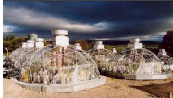
Pivotal to the success and validity of their research has been a suite of 20 Solardome® glasshouses. These 4.5m/15ft diameter domes have been particularly important in enabling large-scale experiments to be carried out on trees and other perennial species which are grown under natural light and ambient temperatures and can be exposed to closely controlled pollution regimes for several consecutive seasons.
